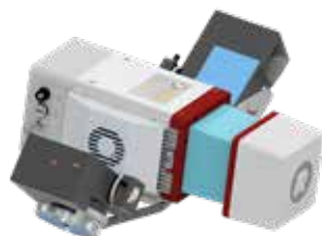
with two Sony Alpha 6000 cameras (oblique mount)
